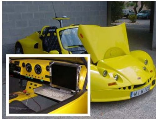
Fig. 2. Test vehicle prototype based on a roadster Comarth S1-50.
