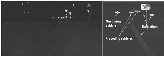
Fig. 3. Left–Middle : nighttime scene imaged with high beams off and on, respectively. Notice how clear is the presence of close poles and traffic signs because of the reflection of the light emitted by the high beams of the car hosting the camera. Right : the energy level of these reflections in the image is equal or higher than the one of mid to far distance head and tail lights of other vehicles.
