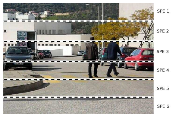
Fig. 5. Fragmentation Approach. A single image is fragmented into same sized pieces. Each piece is then sent to one different SPE.
