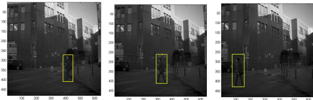
Fig. 7. Snapshots of the scene: the detected pedestrian is crossing the road.
